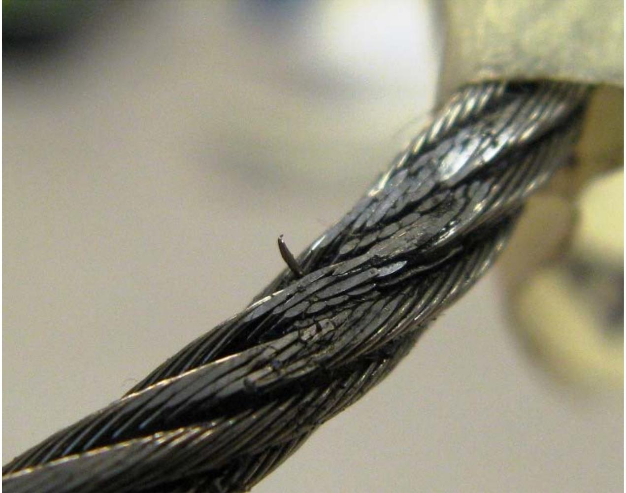
**Cessna 172S, Frayed Aileron Cable, ATA 2710**
