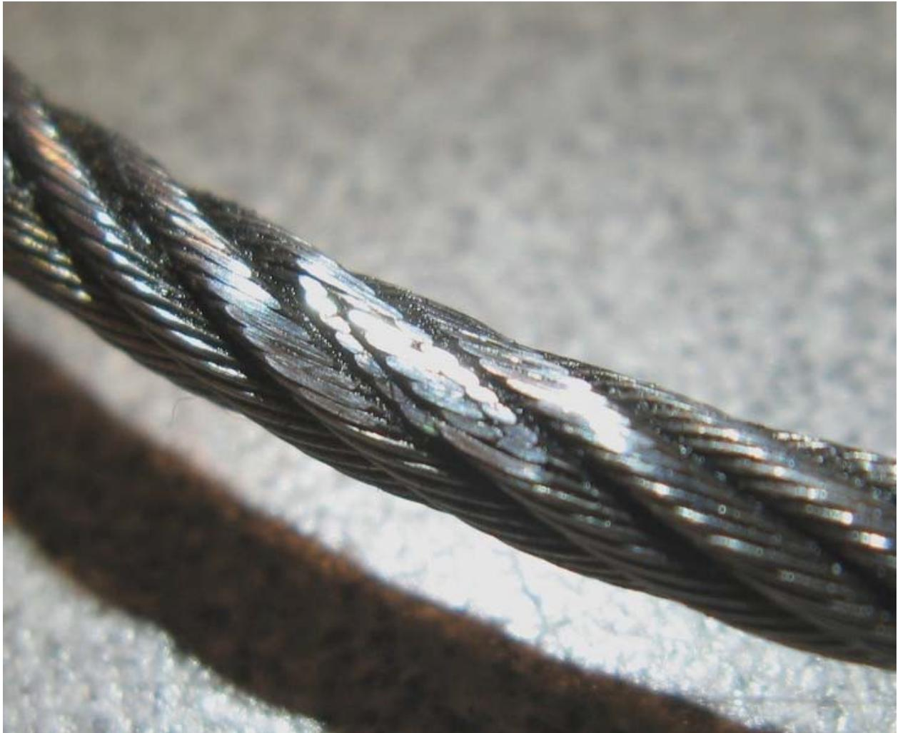
**Cessna 172S, Frayed Aileron Cable, ATA 2710**
